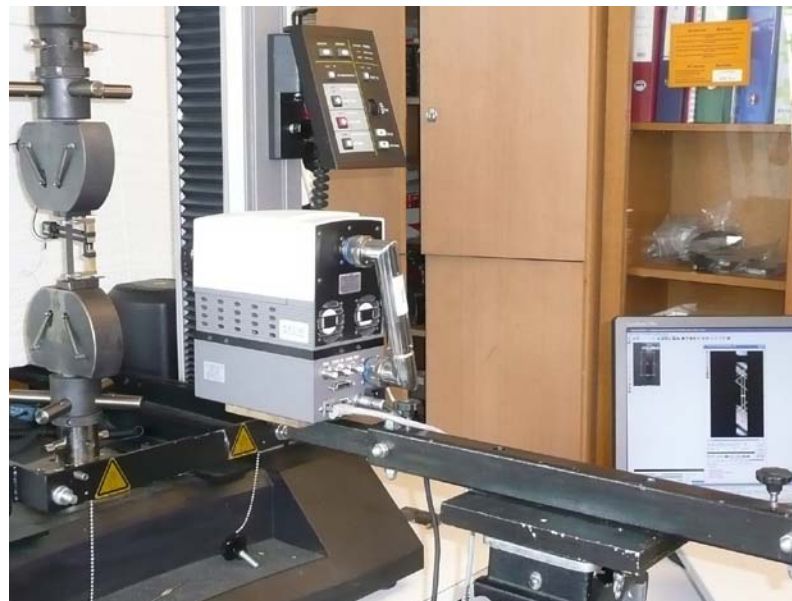
Fig. 1. Photograph of TiNi SMA specimen with mechanical extensometer in grips of Instron testing machine, Flir Phoenix infrared camera and temperature distribution image of localized martensite transformation
